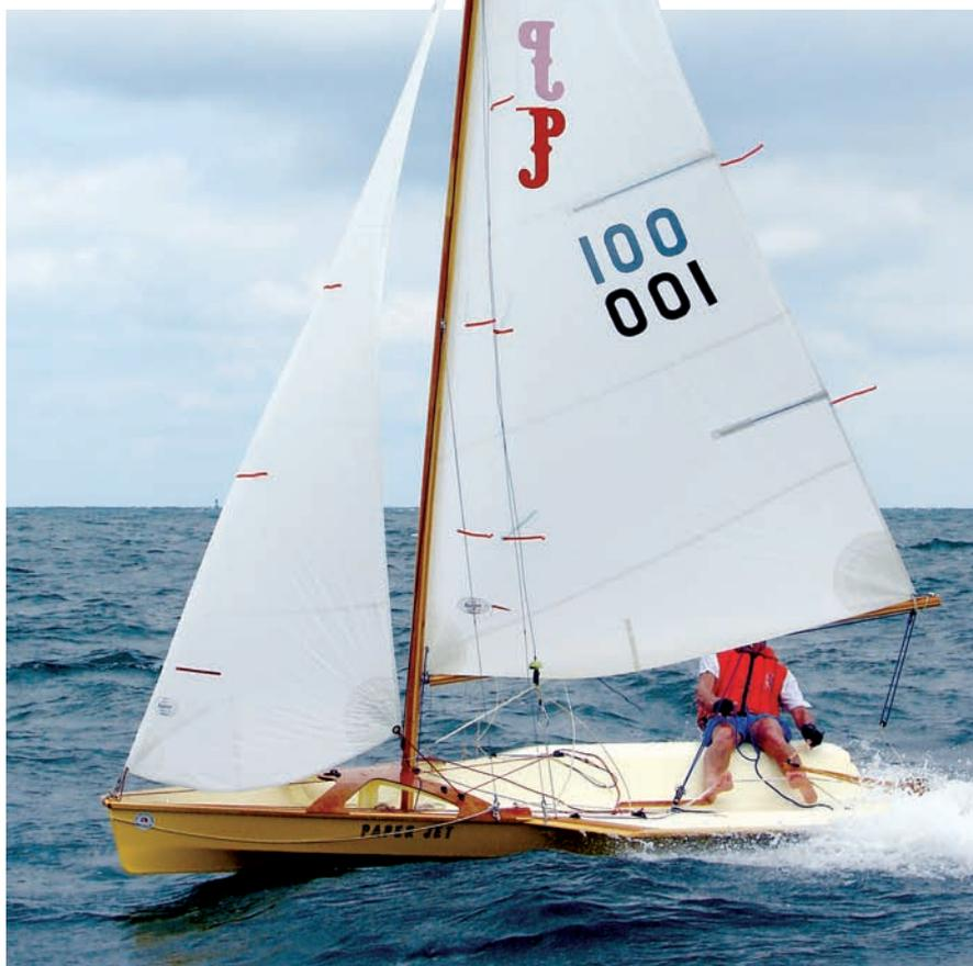
Dudley Dix's Paper Jet 14 (4.1m) at speed under her standard rig. The white upper section of the mast is a carbon fiber sleeve that can be easily replaced by a taller version with additional rigging for the large, high-performance, "turbo" setup. (See the rig options on the next page.)
